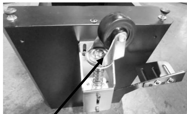
Mobility front wheel screwed onto the shaft
