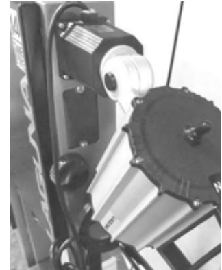
Light fitted in position
