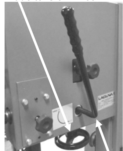
Quick action blade tension lever (activated)
