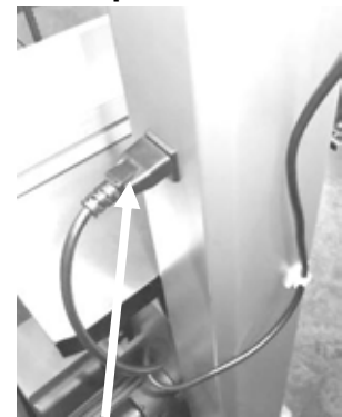
Light plugged into 110v socket
