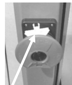
Start/stop with safety removed
