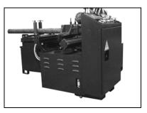
The base is the structure supporting the saw bow (the bow pivot point and respective blocking system), the vise, the rollers, the feeding system, and coolant system.
