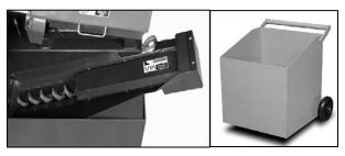
The chip auger automatically starts during a cutting cycle. It is also equipped with anti-jamming device to protect the hydraulic motor. The chip auger conveys chips to the chip cart. Then the cart can be easily wheeled away for waste removal.
