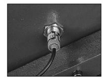
This machine is equipped with automatic power shut-off safety device to prevent any further damage when a blade has been broken. This magnetic switch senses the movement of the blade flywheel. When the blade is broken or loose in tension the flywheel does not move.
