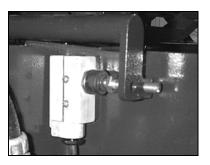
The forward limit switch function as stops for the shuttle vise. Two similar switches are positioned on the hydraulic cylinder of the saw bow to limit the saw bow stroke.
