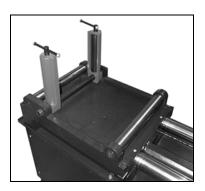
The rollers assist the machine by giving support to long material while allowing the material to glide smoothly during material feeding.
