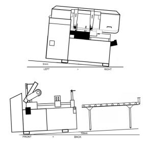
Caution: All leveling bolts should support the weight the machine evenly
