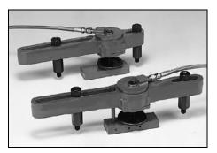
Nestling clamps are used for bundle cutting operations. They vertically press down the material allowing the grouping of many small diameter work pieces. This is efficient for cutting many small, equally sized pieces. These clamps are hydraulically operated.
