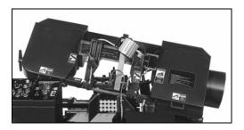
Machine parts consisting of drive members (gear motor or variable speed motor, flywheels), tightening and guide (blade tightening slide, blade guide blocks) of tool.
