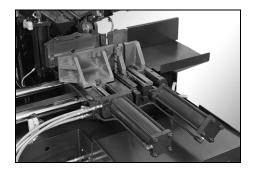
This machine requires the use of two vises to perform the automatic feed operation. The vise system consists of a stationary bench vise with a slot for three phase clamping, and a shuttle vise for feeding work material. The shuttle vise has a floating system that allows it to clamp and feed irregular pieces without binding.
