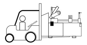
Unpack you machine carefully, and use a crane or forklift to set it in position. If a crane is used to lift the machine, attach the lifting cable carefully to the machine. Sufficient space should be left around the machine to allow safe handling of materials, inspection, and maintenance operations. Take precautions to choose a location that will keep the machine free of vibration and dust caused by other machinery.
