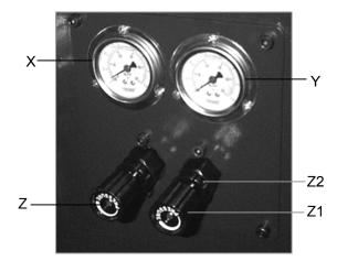
Located just below the gauges are the pressure adjuster knobs. They allow for the reduction of hydraulic pressure or clamping force. The normal pressure for each vise is set at 28kgs/cm<sup>2</sup>. This is good for most solid firm materials, which require 28-30kgs/cm<sup>2</sup>. For softer, hollow, or pipe materials using 15-20kgs/cm<sup>2</sup> is good. Different materials may require different clamping force, so the vise hydraulic pressure is easily changed.
