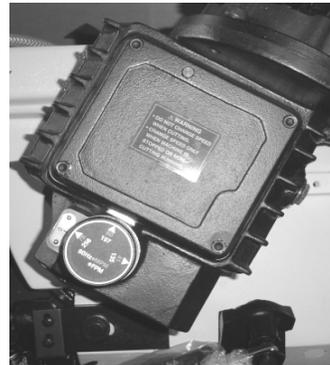
\*\*\*Please make sure the oil of Gear Box is between 950cc ~ 1000cc to ensure proper operation of the gearbox.
