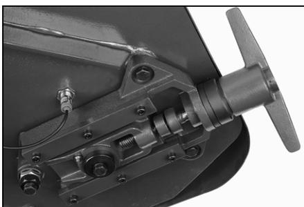
This control is a manual rotation device to set and release the blade tension.
