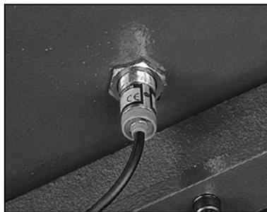
This machine is equipped with automatic power shut-off safety device to prevent any further damage when a blade has been broken. This magnetic switch senses the movement of the blade flywheel. When the blade is broken or loose in tension the flywheel does not move.
