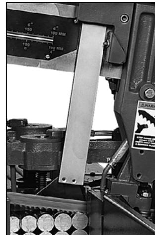
A device that speeds up the operation time by allowing the saw bow to descend quickly and then slow to the cutting pressure rate just before blade touches the workpiece.
